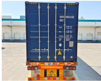
Figure 4-3: Closed container with markings
